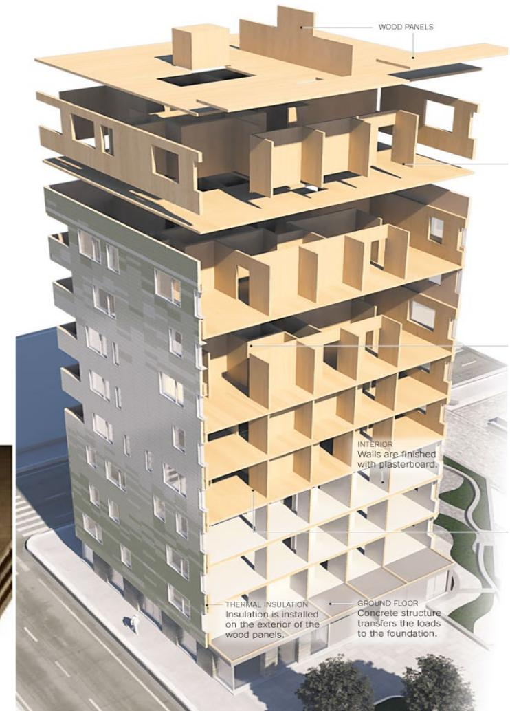
Use CLT panels and the main structural components, walls and floors of the building.
